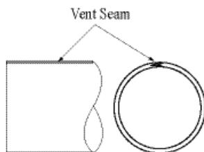
**Notice:** Make sure that the seam of the vent pipe in horizontal runs is toward the top of the installation (see Figure above).
